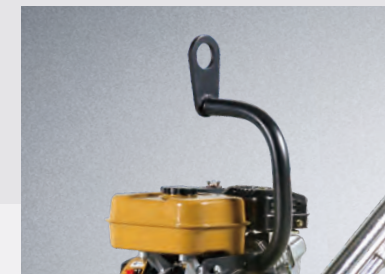
Lifting eyelet another method for easy transportation.
