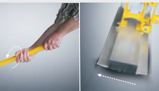
Turning the handle to the right, to make the blade inclines forward, pushing and spreading the concrete.
